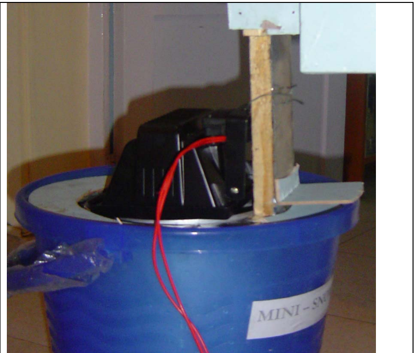
This is how the 300 watt halogen bulb sits comfortably over the rim of the drum
