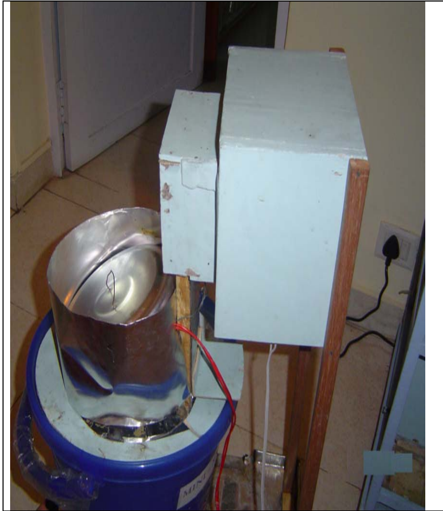
The bulb is lightly encased in an aluminium roll and covered with the lid of the drum to deflect humidified hot air into the grooves.
