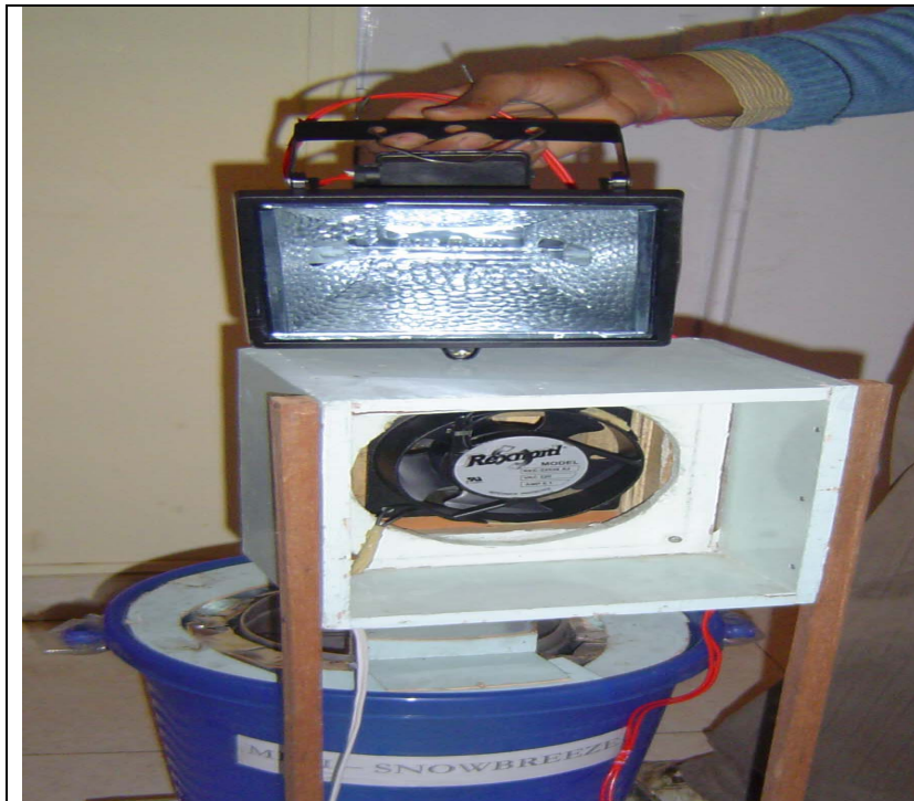
In winter a 300 watt halogen bulb is inverted upon the rim of the drum which is half filled with water to serve as a room heater
